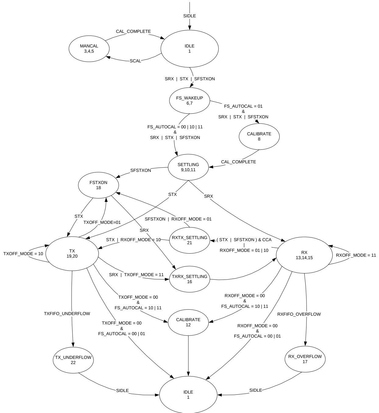
Figure 55: Complete Radio Control State Diagram
