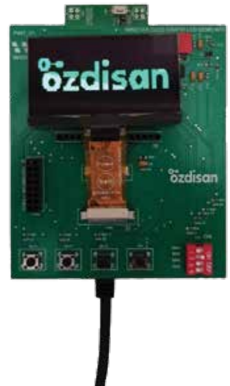
Graphic OLED example (128x64);
