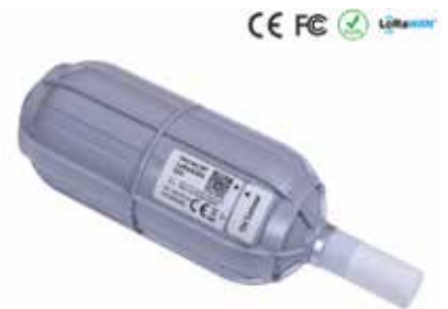
SeeedStudio LoRaWAN Air Pressure Sensor
