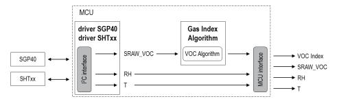
**Figure 7** Schematic of the driver and Gas Index Algorithm implementation on a microcontroller.
