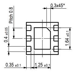
Figure 13 Package outline drawing of the SGP40. Dimensions are given in millimeters.
