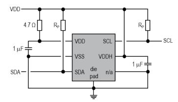
Figure 5 Typical application circuit.
