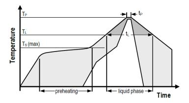
**Figure 15** Soldering profile according to JEDEC standard. Recommended conditions are  $T_P = 245$ °C and  $t_P \le 30$  s for Pb-free assembly,  $T_L < 220$ °C and  $t_L < 150$  s. Ramp-up rate < 3°C s<sup>-1</sup> and ramp-down rate < 4°C s<sup>-1</sup>.
