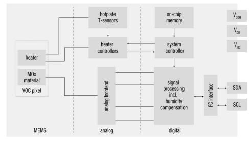
Figure 1 Functional block diagram of the SGP40.
