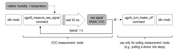
**Figure 6** Process flow for performing a raw signal measurement with the SGP40. For enabling on-chip humidity compensation, current relative humidity and temperature values have to be supplied as part of the measurement command.
