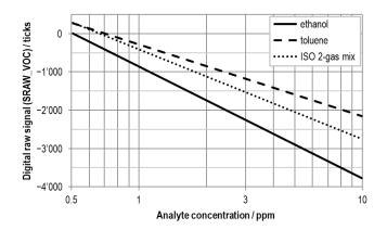
**Figure 2** Typical sensor response to various VOCs normalized to 500 ppb of ethanol. ISO 2-gas mix according to ISO16000-29 is composed of n-octane and m-xylene in a molar ratio of 53:47. Data were recorded at 25 °C and 50 % RH and a power supply of VDD of 3.3 V.
