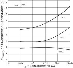
Fig. 6 Drain-Source On-Resistance vs. Drain-Current
