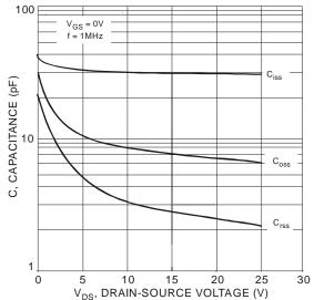
Fig. 10 Capacitance vs. Drain-Source Voltage
