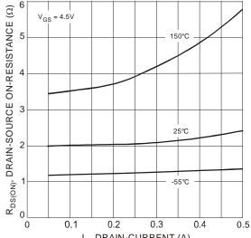
${\rm I_D}, {\rm DRAIN\text{-}CURRENT}$  (A) Fig. 7 Drain-Source On-Resistance vs. Drain-Current
