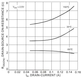
Fig. 5 Drain-Source On-Resistance vs. Drain-Current
