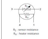
Fig 1d. Equivalent circuit
