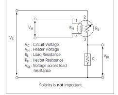
Fig 2. Standard circuit
