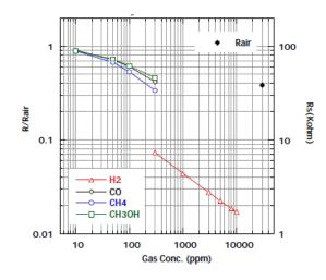
Fig 3. Sensitivity characteristics
