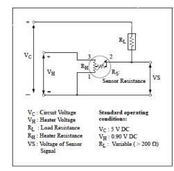
Fig 2. Standard circuit
