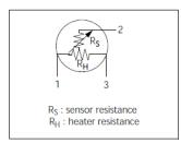
Fig 1d. Equivalent circuit
