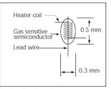
Fig 1a. Sensing element
