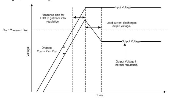
Figure 8-2. Start-Up Into Dropout
