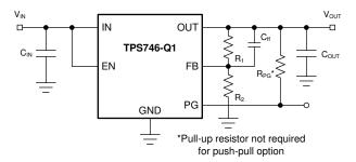
Figure 8-1. Adjustable Operation
