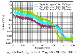
Figure 6-44. Output Spectral Noise Density vs Frequency
