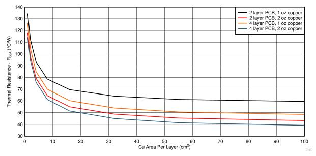
Figure 8-5.  $R_{\theta JA}$  versus Cu Area for the WSON (DRV) Package
