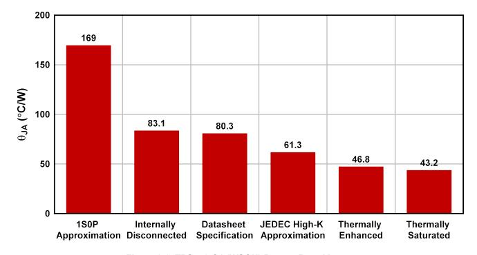
Figure 8-8. TPS746-Q1 (WSON)  $R_{\theta JA}$  vs Board Layout
