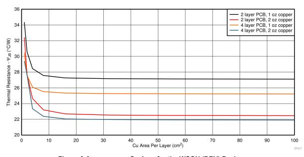
Figure 8-6.  $\psi_{JB}$  versus Cu Area for the WSON (DRV) Package
