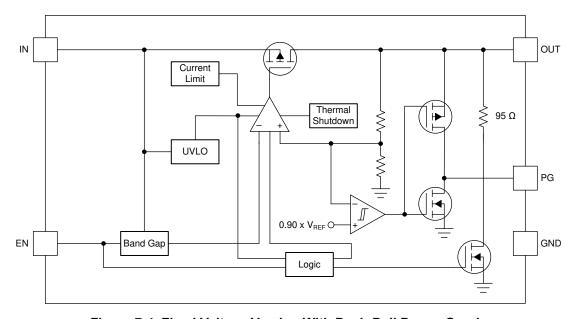
Figure 7-4. Fixed Voltage Version With Push-Pull Power-Good
