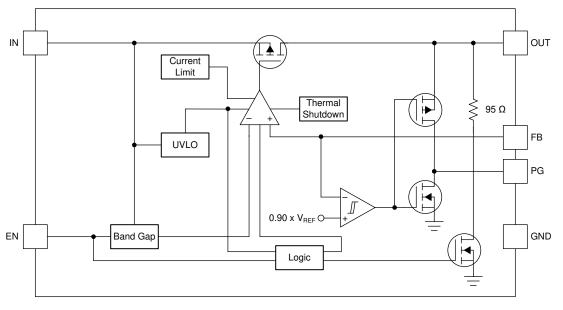
Figure 7-2. Adjustable Version With Push-Pull Power-Good
