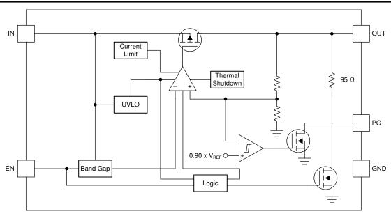
Figure 7-3. Fixed Voltage Version With Open-Drain Power-Good
