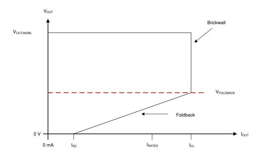
Figure 7-5. Foldback Current Limit
