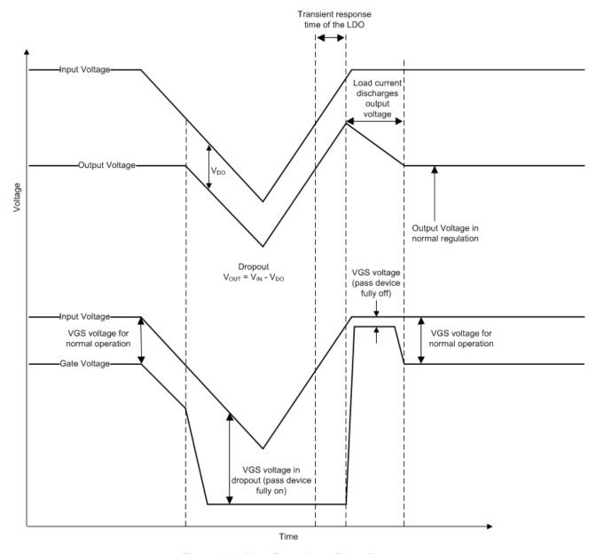
Figure 8-3. Line Transients From Dropout
