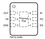
Figure 5-1. DRV Package, 6-Pin Adjustable WSON (Top View)
