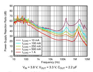
Figure 8-10. PSRR vs Frequency and I<sub>LOAD</sub>
