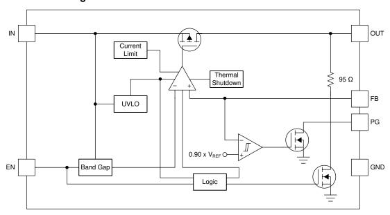
Figure 7-1. Adjustable Version With Open-Drain Power-Good
