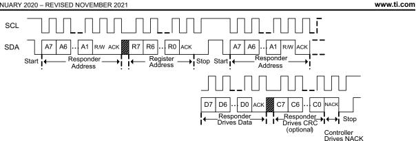
Figure 14-3. I<sup>2</sup>C Read Without Repeated Start
