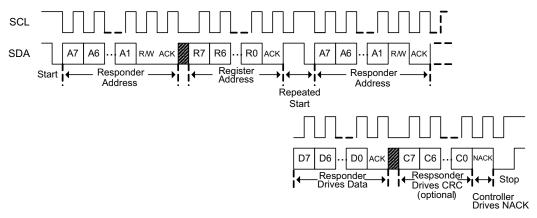
Figure 14-2. I<sup>2</sup>C Read with Repeated Start
