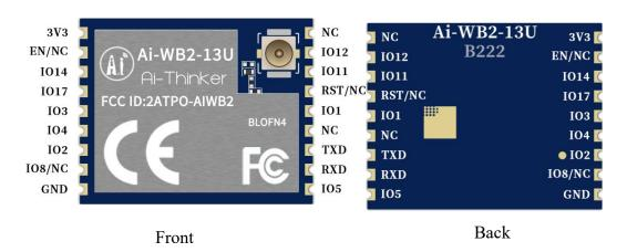
Figure 6 Schematic diagram of module pins
