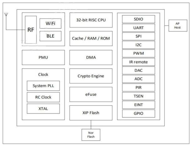
Figure 1 Main chip block diagram
