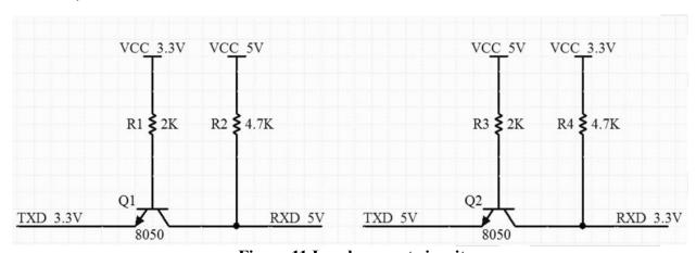
Figure 11 Level convert circuit
