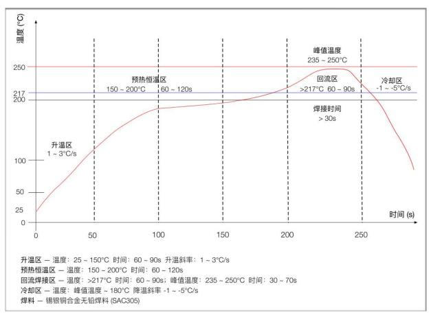
Figure 12 Reflow welding diagram
