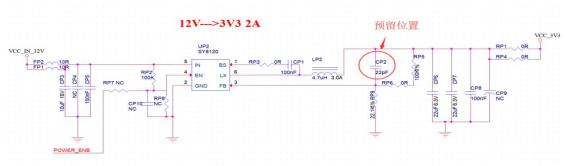
Figure 10 DC-DC step-down circuit diagram
