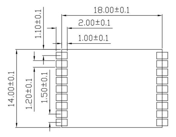
Figure 9 Recommend PCB footprint size
