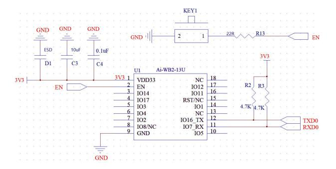
Figure 8 Application circuit diagram
