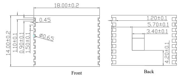
Figure 4 Dimension diagram
