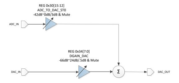
Figure 5 DAC Path Digital Mixer with Sidetone
