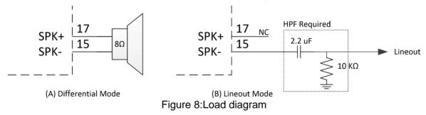
With the above sequence,the rise time is a function of  $C_{ext}$  and can be approximated by the equation  $t_{rise} = 1 + 27*10^{4*}C_{ext}$  (example: for  $C_{ext} = 2.2 uF$ ,  $R_L = 10 k$ , the rise time is ~ 1.6 secs).
