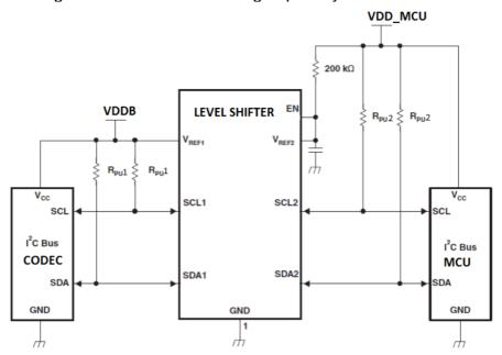
Figure 13 Typical I2C level shifter circuit
