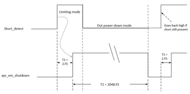
Figure 6 Speaker driver short-circuit protection timing
