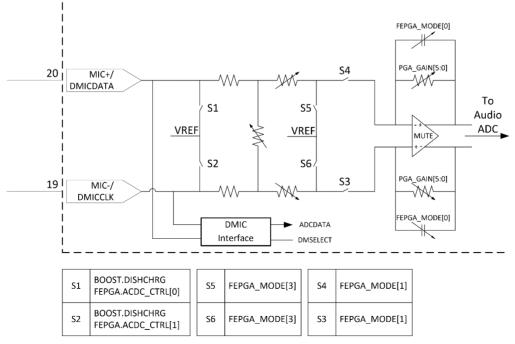
Figure 1: Microphone Input Block Diagram with Registers
