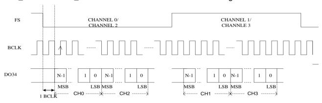
Figure 24 TDM I2S Audio Format
