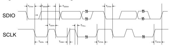
Figure 17 Two-wire Control Mode Timing
