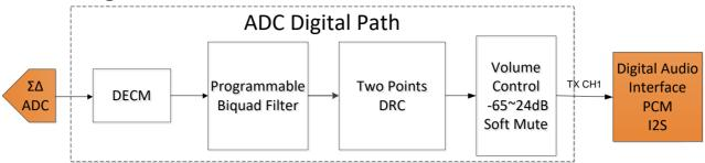
Figure 2 ADC Digital Path
