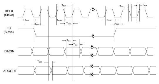
Figure 28 Audio Inteface Mode Slave Timing
