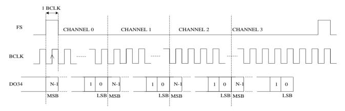
Figure 26 TDM PCMB Audio Format
