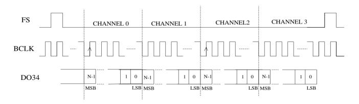
Figure 27 TDM PCM Offset Audio Format
