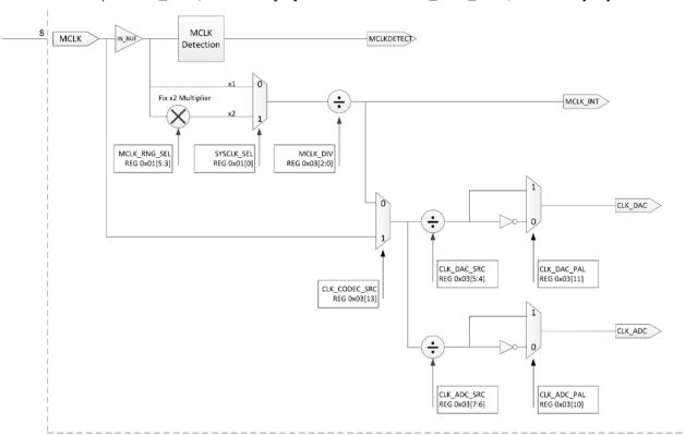
Figure 9 NAU88L11 MCLK and Clock Distribution
