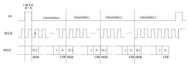
Figure 25 TDM PCMA Audio Format
