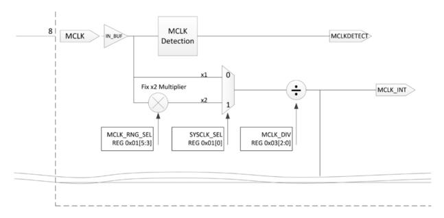
Figure 8 NAU88L11 Clock Detection
