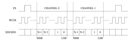
Figure 23 PCM Time Slot Audio Interface
