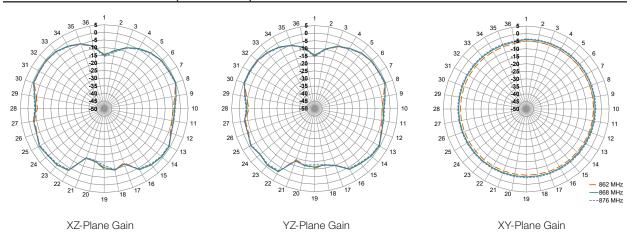
Figure 8. ANT-868-OC-LG Radiation Patterns
