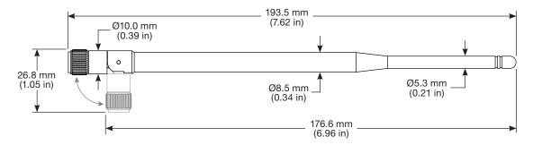
Figure 1. OC-LG Antenna Dimensions
