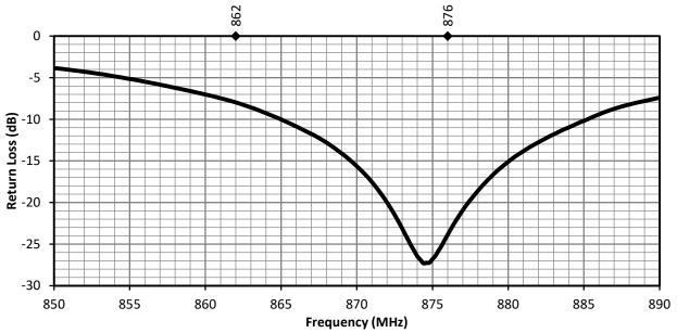
Figure 4. ANT-868-OC-LG Return Loss
