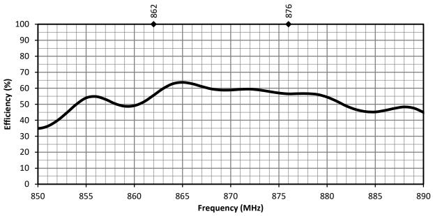
Figure 7. ANT-868-OC-LG Antenna Efficiency
