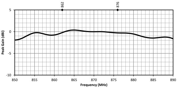
Figure 5. ANT-868-OC-LG Peak Gain
