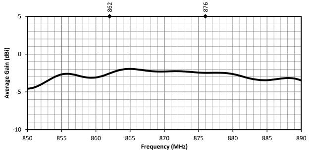
Figure 6. ANT-868-OC-LG Antenna Average Gain
