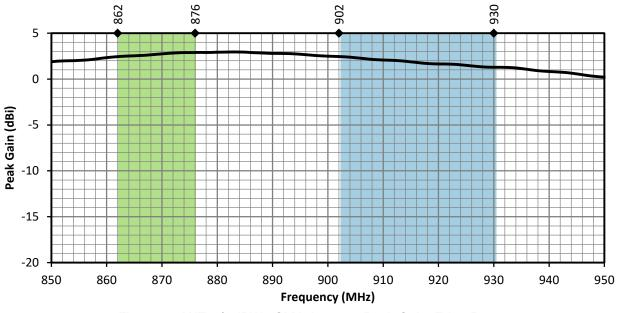
Figure 6. ANT-8/9-IPW1-SMA Antenna Peak Gain, Edge Bent
