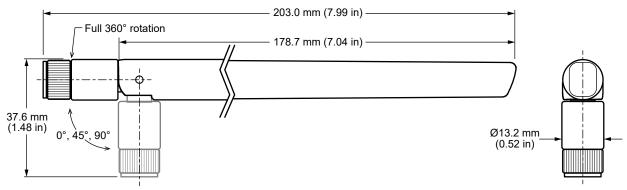
Figure 1. ANT-8/9-IPW1-SMA Antenna Dimensions
