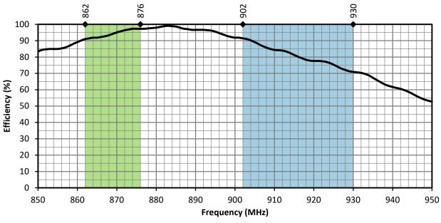
Figure 8. ANT-8/9-IPW1-SMA Antenna Radiation Efficiency, Edge Bent
