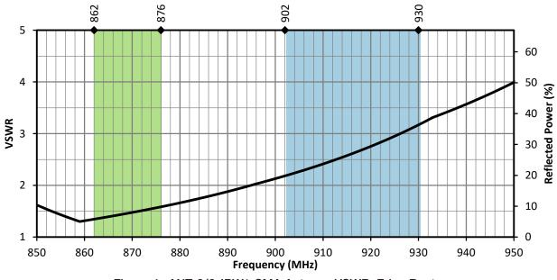
Figure 4. ANT-8/9-IPW1-SMA Antenna VSWR, Edge Bent
