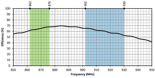
Figure 15. ANT-8/9-IPW1-SMA Antenna Radiation Efficiency, Straight
