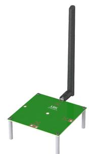
Figure 3. ANT-8/9-IPW1-SMA at Edge of Ground Plane, Bent 90 Degrees (Edge Bent)
