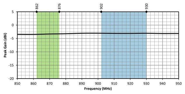
Figure 4. 8/9-FPC Antenna Peak Gain with Frequency Band Highlights
