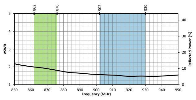
Figure 2. 8/9-FPC Antenna VSWR with Frequency Band Highlights
