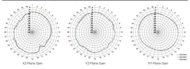
Figure 7. Radiation Patterns for ANT-8/9-FPC-UFL-100 Antenna
