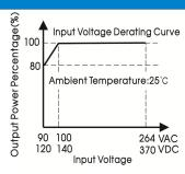
Note: 1. With an AC input voltage between 90 -100VAC and a DC input between 120-140VDC the output power must be derated as per the temperature derating curves;
