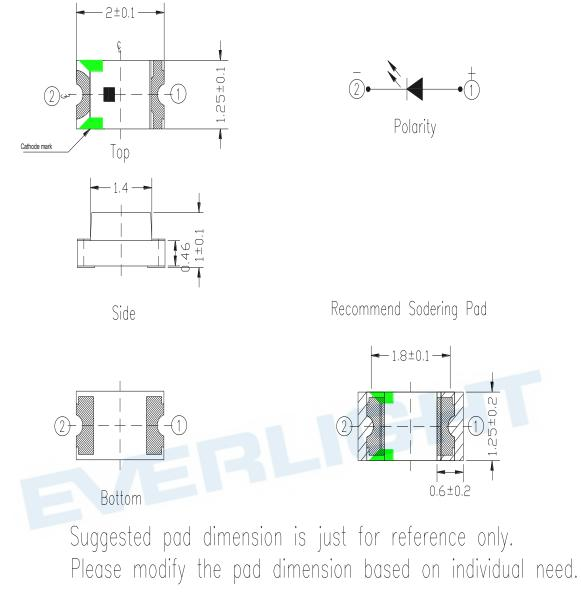
Note: Tolerances unless mentioned  $\pm 0.1$ mm. Unit = mm
