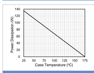
Fig.3 Power Derating Curve
