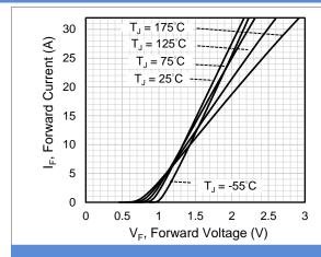
**Fig.1 Forward Characteristics**
