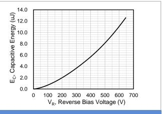
Fig.6 Capacitance Stored Energy
