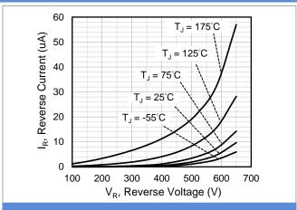
Fig.2 Reverse Characteristics
