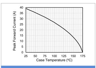
**Fig.4 Current Derating Curve**
