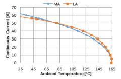
Figure 20: Maximum Continuous Current at a Given T<sub>A</sub>
