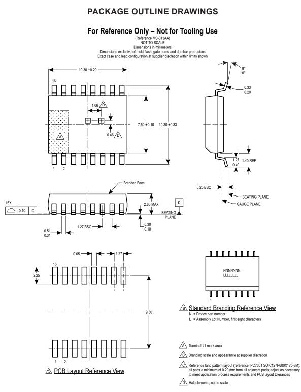
Figure 22: Package MA, 16-Pin SOICW
