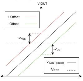
Figure 7: Offset (V<sub>OE</sub>) Between V<sub>IOUT</sub> and V<sub>REF</sub>
