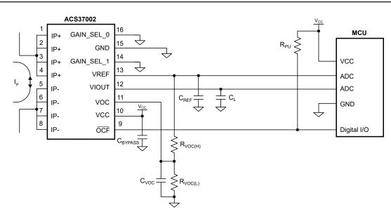
Figure 1: Typical Bidirectional Application Showing 00 Gain Select Configuration. For more application circuits, refer to the Application and Theory section.
