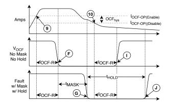
Figure 13: General Fault Timing. Note: the MASK and HOLD functionality are independent of each other
