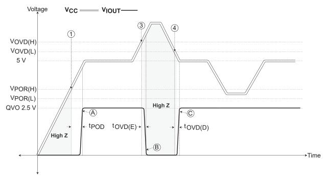
Figure 6:  $t_{POD}$  and  $t_{OVD(E/D)}$  with  $R_L$  = Pull-Up
