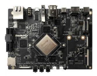
Support TensorFlow / Caffe / Mxnet Support 8bit/16bit operation Up to 3.0TOPs
