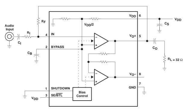
Figure 2. SE Mode Test Circuit
