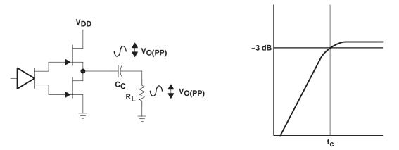
Figure 49. Single-Ended Configuration and Frequency Response
