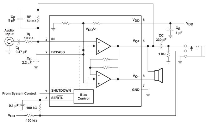
Figure 51. TPA711 Application Circuit
