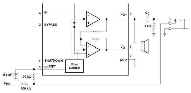
Figure 52. TPA711 Resistor Divider Network Circuit
