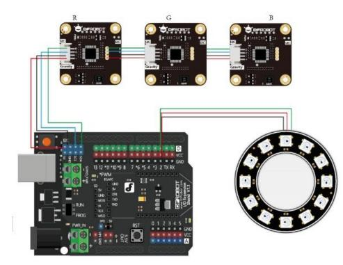
Use Case Diagram (Control RGB LED by three encoders)
