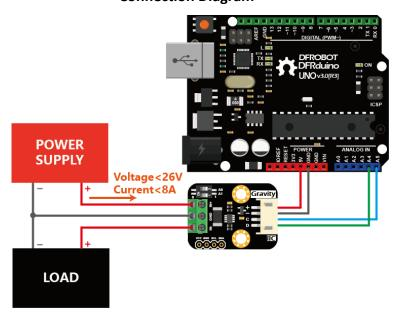
Gravity: I2C Digital Wattmeter Connection Diagram (Arduino UNO)
