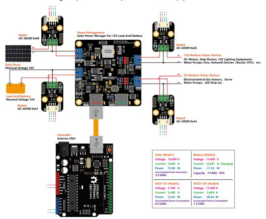
Monitor the power consumption of the solar panel, battery and outputs of a solar system
