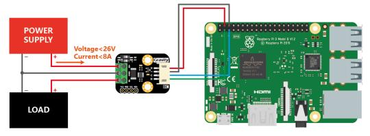
Gravity: I2C Digital Wattmeter Connection Diagram (Raspberry Pi 3B)
