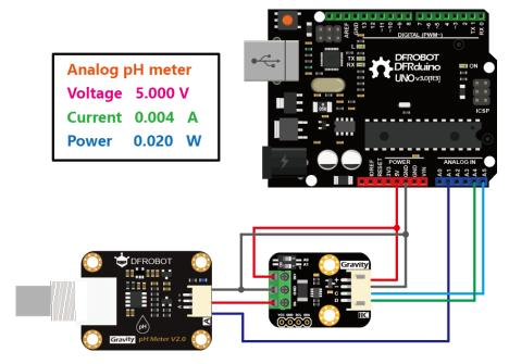
Measuring the power consumption of the Gravity: pH meter
