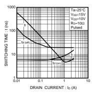
Fig.2 Switching Characteristics
