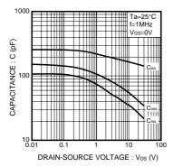
Fig.1 Typical Capacitance vs. Drain-Source Voltage
