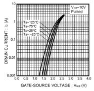
Fig.4 Typical Transfer Characteristics
