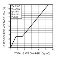
Fig.3 Dynamic Input Characteristics
