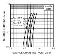
Fig.6 Source Current vs. Source-Drain Voltage
