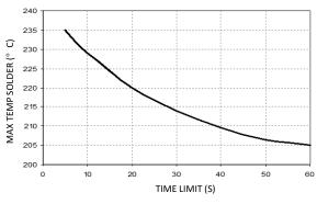
Figure 22. Time Limit,  $T_{\textrm{lim}},$  Curve Above 205°C Reflow.
