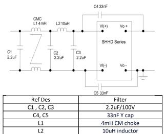
Figure 18 Suggested Configuration for EN55032 Class
