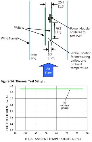
Figure 15. Output Current Derating for the Open Frame SHHD001A3B in the Transverse Orientation; Airflow Direction from Vin(-) to Vin(+); Vin = 24V.
