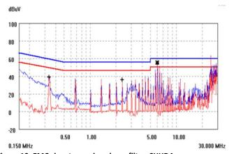
**Figure 19. EMC signature using above filter, SHHDA.** For further information on designing for EMC compliance, please refer to the FLTR100V10 data sheet (FDS01-043EPS).
