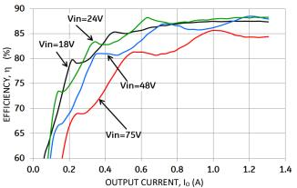
Figure 1. Converter Efficiency versus Output Current.
