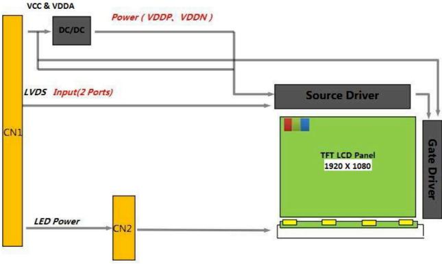
Figure 1: Function Diagram
