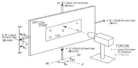
Figure 8: Measurement Set Up
