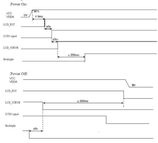
Note 1: When STBYB rise high, it take 10 display data frame for internal power step up.
