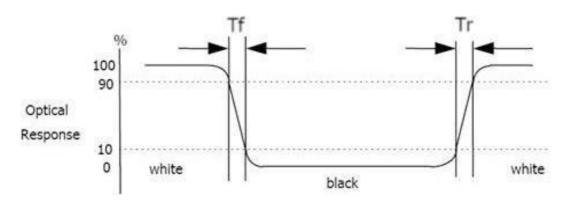
Figure 10: Response Time Testing
