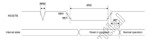
Figure 6: Reset timing
