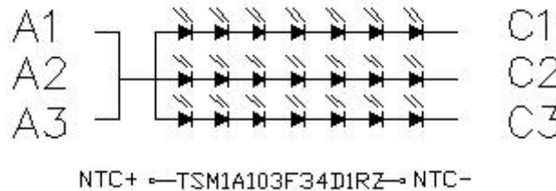
Note 2: The “LED life time” is defined as the module brightness decrease to 50% original brightness at Ta=25°C and I<sub>L</sub> =95mA (each LED). The LED lifetime could be decreased if operating I<sub>L</sub> is larger than 120 mA.
