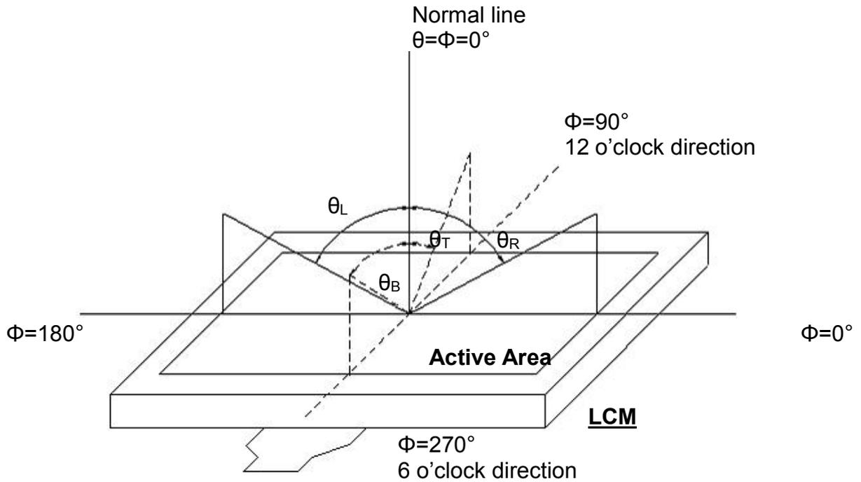
Fig. 4-2 Definition of viewing angle
