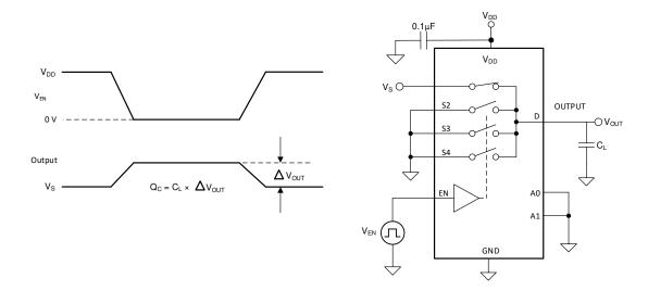
Figure 13. Charge-Injection Measurement Setup
