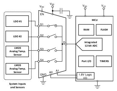
Figure 18. Multiplexing Signals to Integrated ADC
