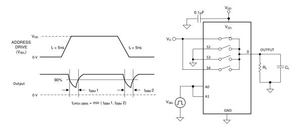
Figure 11. Break-Before-Make Delay Measurement Setup
