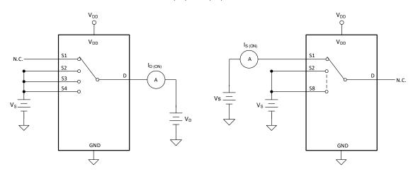
Figure 9. On-Leakage Measurement Setup
