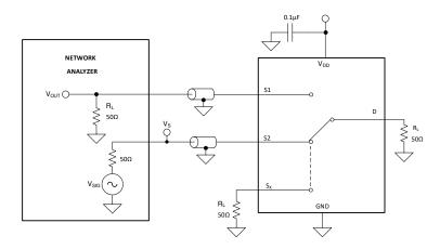
Figure 15. Crosstalk Measurement Setup
