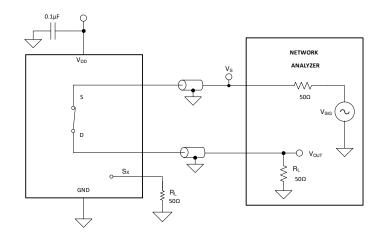
Figure 16. Bandwidth Measurement Setup
