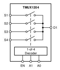
Figure 17. TMUX1204 Functional Block Diagrams
