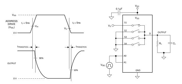
Figure 10. Transition-Time Measurement Setup
