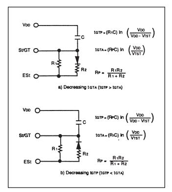
Figure 5. Guard Time Adjustment
