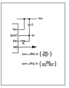
Figure 4. Basic Steering Circuit
