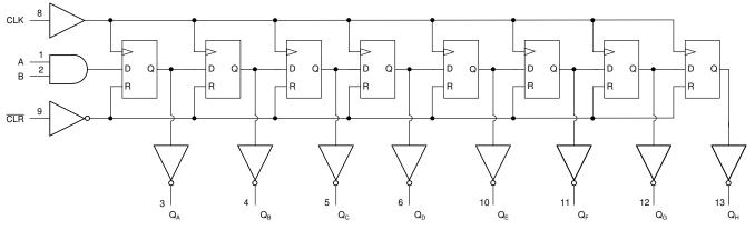
Figure 7-1. Functional Block Diagram
