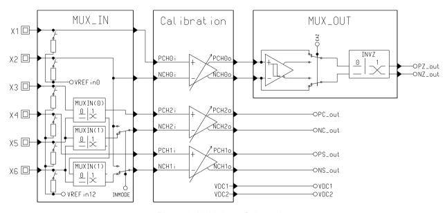
Figure 6: Multiplexer Schematics
