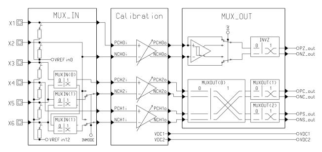
Figure 7: Multiplexer Schematics
