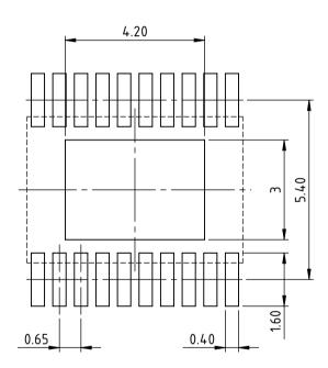
All dimensions given in mm. Tolerances of form and position according to JEDEC MO-153
