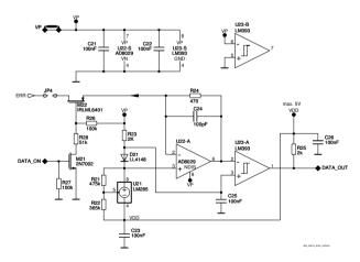
Figure 2: Example circuit for the decoding and conversion of the current-modulated signals to logic levels.
