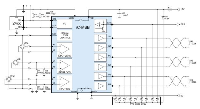
Figure 11: Example circuit for safety-related applications with iC-MSB<sup>SAFETY</sup>.
