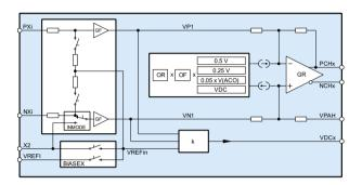
Figure 3: Signal conditioning input circuit.
