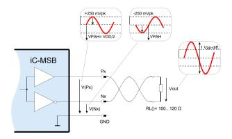
Figure 10: Output amplitude and offset according to Elec. Char. 502 and 503.
