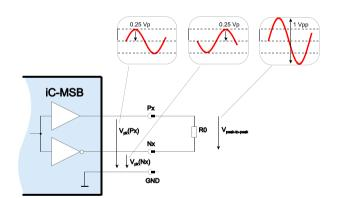
Figure 8: Definition of 1 Vpp signal. Termination R0 must be high-ohmic during all *Test* and *Calibration* modes.
