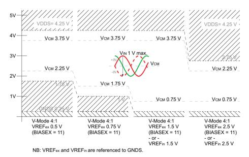
Figure 5: Permissible common mode range for voltage input 4:1 in dependancy to the reference voltage.
