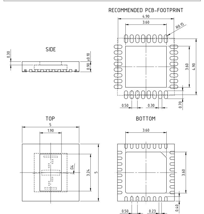
All dimensions given in mm. Tolerances of form and position according to JEDEC MO-220. Positional tolerance of sensor pattern:  $\pm 70 \mu m$  /  $\pm 1^{\circ}$  (with respect to center of backside pad). G4: radius of chip center (refer to the relevant encoder disc and code description). Maximum molding excess  $\pm 20 \mu m$  /  $-75 \mu m$  versus surface of glass/reticle.
