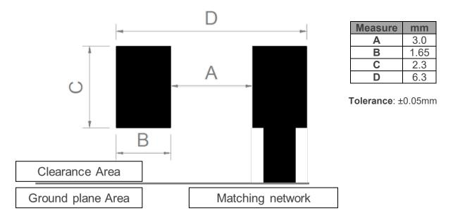
Footprint dimensions for the ONE mXTEND<sup>™</sup> (NN02-201) antenna booster.
