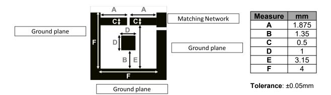
Footprint dimensions for the NANO mXTEND™ (NN02-101) antenna booster (in the middle).
