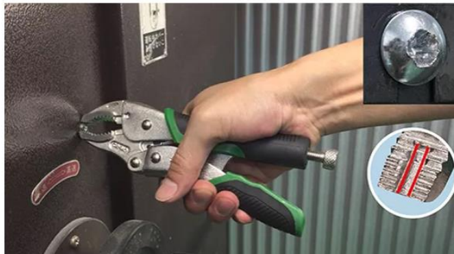
Step 4 : Squeeze the handles to lock the jaws.
