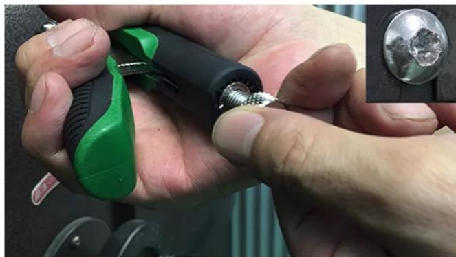
Step 3 : Fasten the adjusting bolt further (half a turn to the right)
