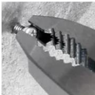
Bite screw head and unfasten it
