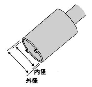
Overall Length (mm)- 150 Handle Diameter ( $\Phi$ mm)- 28 Trusco Part No- 395- 4811 Shaft Length (mm)- 53 Shank Diameter ( $\Phi$ mm)- 8 Mass (g)- 99 Type- Dedicated driver Material (Grip)- Resin Set Contents- Single item Inner Dimensions (mm)-  $\Phi$ 15.8 Outer Dimensions (mm)-  $\Phi$ 20
