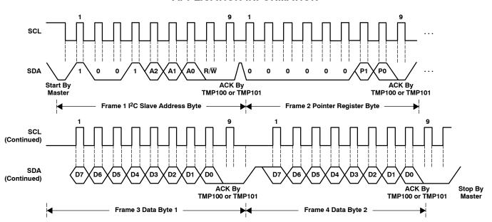
Figure 5. I<sup>2</sup>C Timing Diagram for Write Word Format
