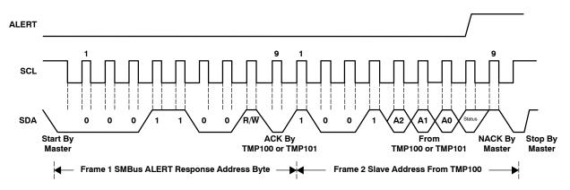
Figure 7. Timing Diagram for SMBus ALERT
