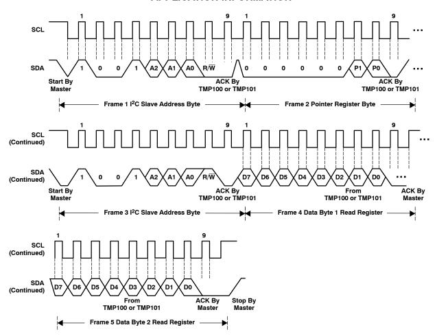
Figure 6. I<sup>2</sup>C Timing Diagram for Read Word Format
