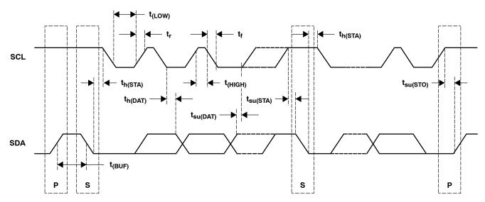
Figure 4. I<sup>2</sup>C Timing Diagram
