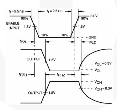
Figure 4. AC Waveforms
