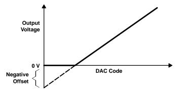
Figure 13. Effect of Negative Offset (Single Supply)
