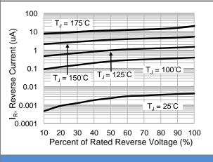
Fig.3 Typical Reverse Characteristics
