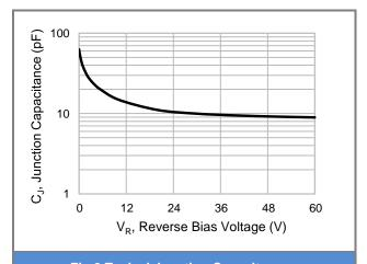
**Fig.2 Typical Junction Capacitance**
