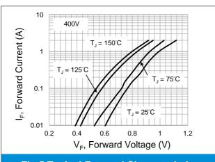
Fig.5 Typical Forward Characteristics
