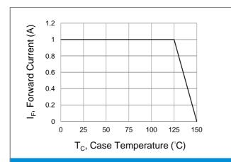
**Fig.1 Forward Current Derating Curve**
