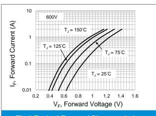
**Fig.6 Typical Forward Characteristics**
