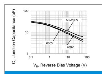
**Fig.2 Typical Junction Capacitance**
