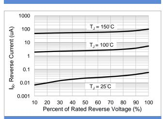
Fig.3 Typical Reverse Characteristics
