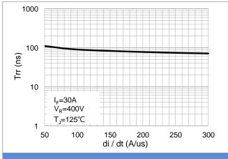
Fig.5 Typical Reverse Recovery Time Versus di/dt
