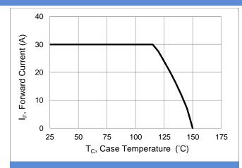
**Fig.1 Forward Current Derating Curve**
