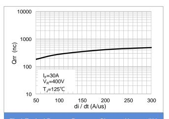
Fig.6 Typical Reverse Recovery Charges Versus di/dt
