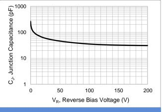
Fig.2 Typical Junction Capacitance
