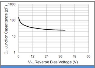
**Fig.2 Typical Junction Capacitance**
