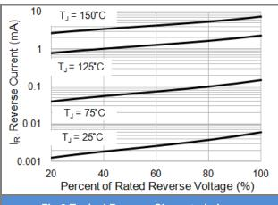
Fig.3 Typical Reverse Characteristics
