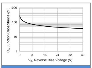
**Fig.2 Typical Junction Capacitance**
