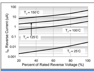
Fig.3 Typical Reverse Characteristics
