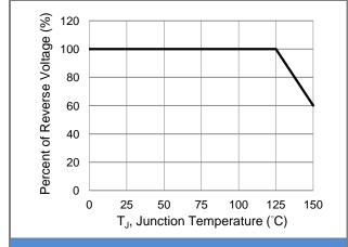
Fig.5 Operating Temperature Derating Curve
