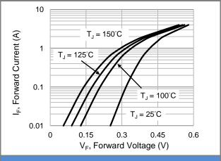
Fig.4 Typical Forward Characteristics
