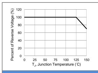
**Fig.5 Operating Temperature Derating Curve**
