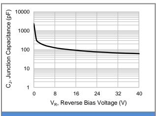
**Fig.2 Typical Junction Capacitance**
