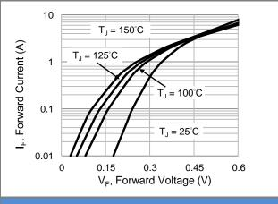
Fig.4 Typical Forward Characteristics
