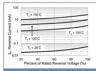
Fig.3 Typical Reverse Characteristics
