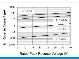
Fig.3 Typical Reverse Characteristics
