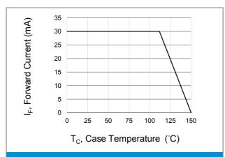
**Fig.1 Forward Current Derating Curve**
