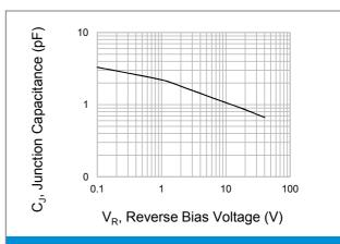
**Fig.2 Typical Junction Capacitance**
