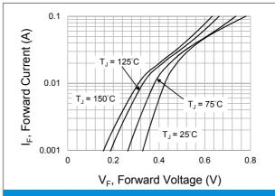
Fig.4 Typical Forward Characteristics
