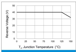
**Fig.5 Operating Temperature Derating Curve**
