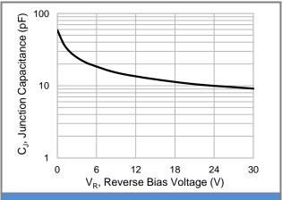
Fig.2 Typical Junction Capacitance
