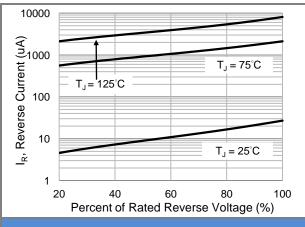
Fig.3 Typical Reverse Characteristics
