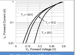
Fig.4 Typical Forward Characteristics
