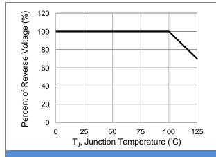
**Fig.5 Operating Temperature Derating Curve**
