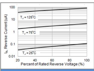
Fig.3 Typical Reverse Characteristics
