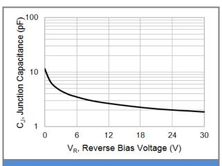
**Fig.2 Typical Junction Capacitance**
