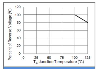
Fig.5 Operating Temperature Derating Curve
