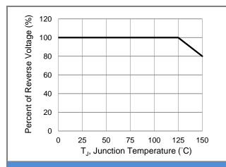
Fig.5 Operating Temperature Derating Curve
