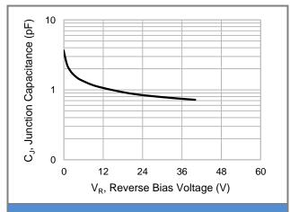
**Fig.2 Typical Junction Capacitance**
