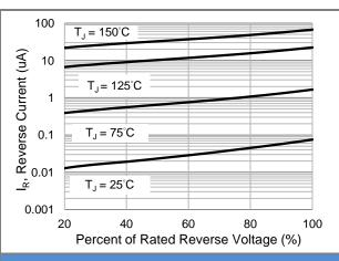
Fig.3 Typical Reverse Characteristics
