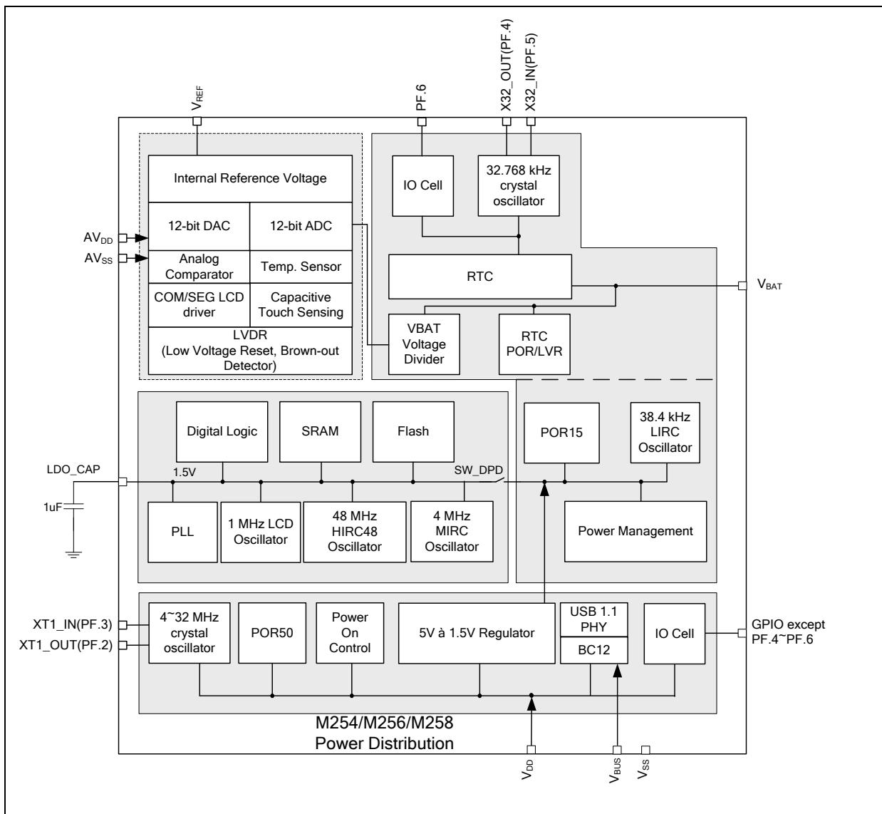
Figure 6.2-6 NuMicro® M254/M256/M258 Series Power Distribution Diagram
