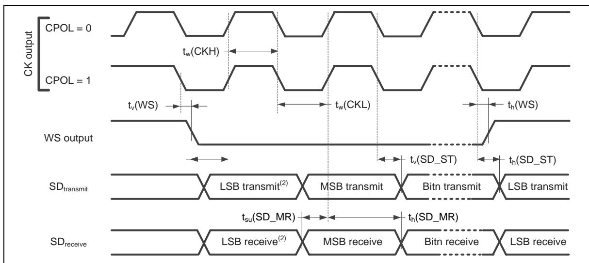
Figure 8.6-3 I<sup>2</sup>S Master Mode Timing Diagram
