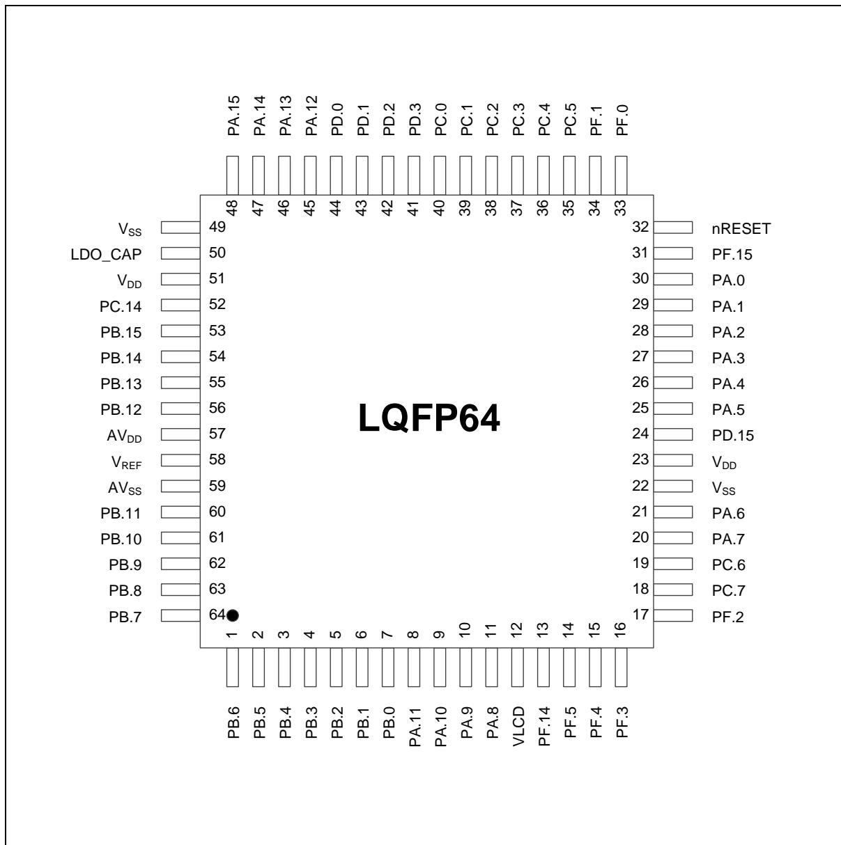
Figure 4.1-2 M254 Series LQFP 64-pin Diagram without V<sub>BAT</sub>
