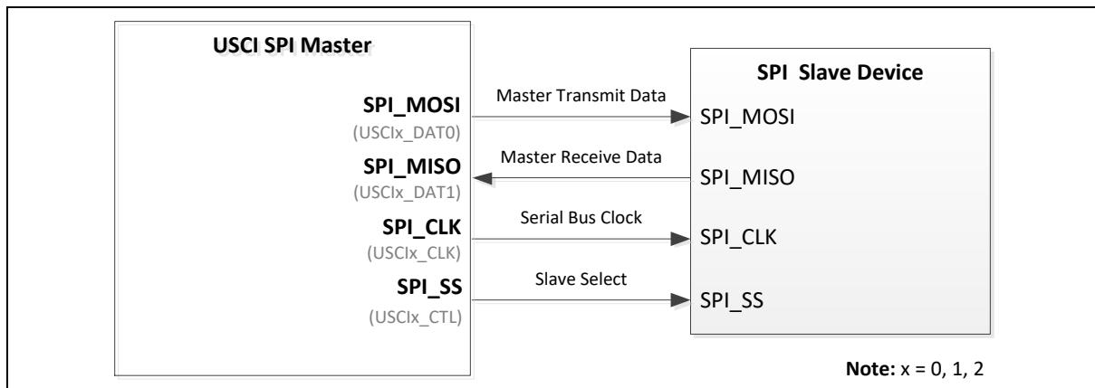
Figure 6.18-1 SPI Master Mode Application Block Diagram
