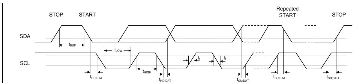
Figure 8.6-5 I<sup>2</sup>C Timing Diagram
