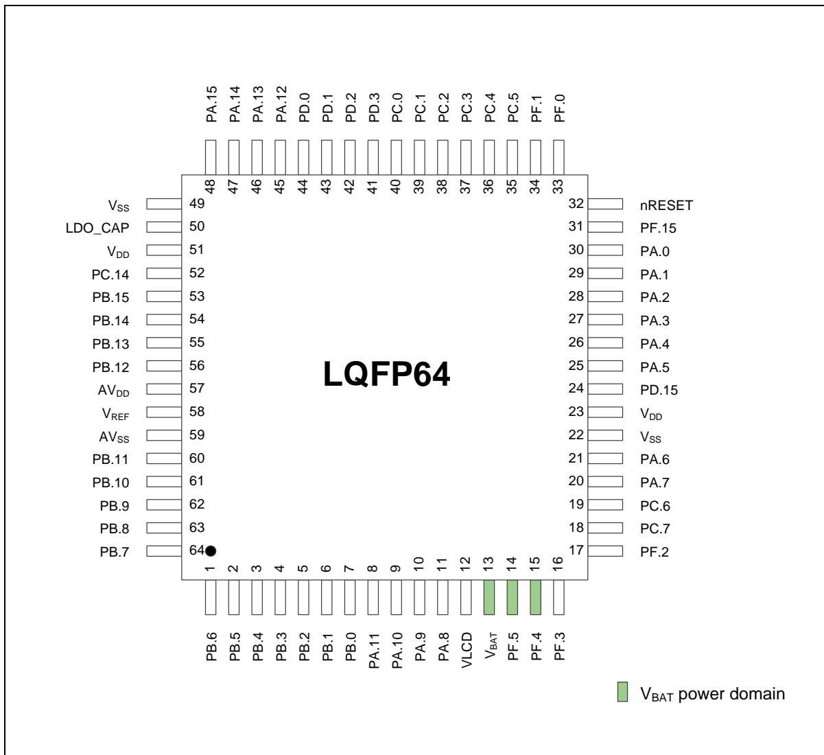
Figure 4.1-3 M254 Series LQFP 64-pin Diagram with V<sub>BAT</sub>
