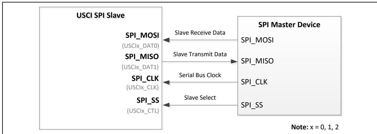
Figure 6.18-2 SPI Slave Mode Application Block Diagram
