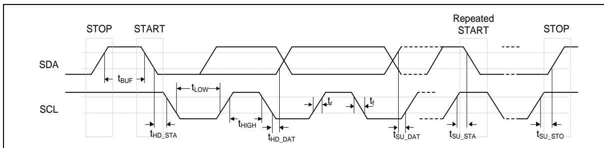
Figure 6.19-1 I<sup>2</sup>C Bus Timing
