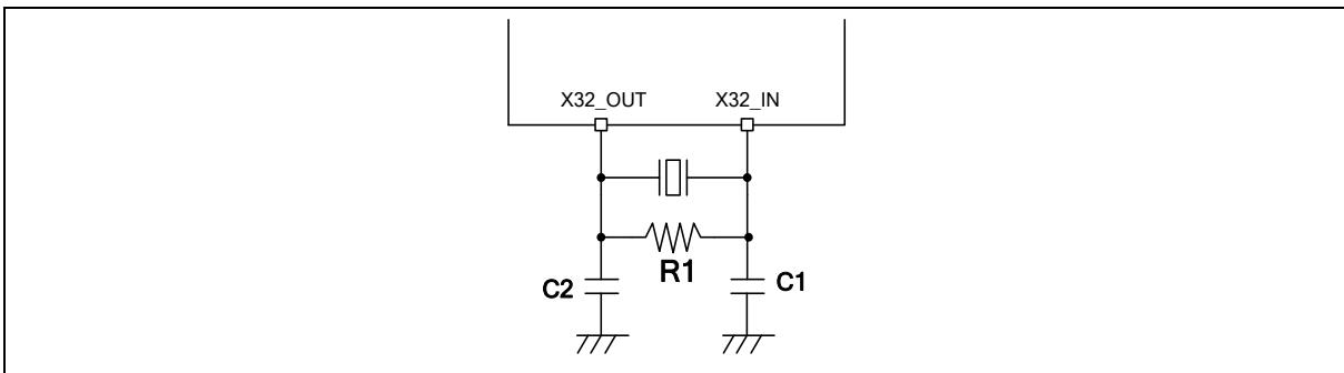
Figure 8.4-3 Typical 32.768 kHz Crystal Application Circuit
