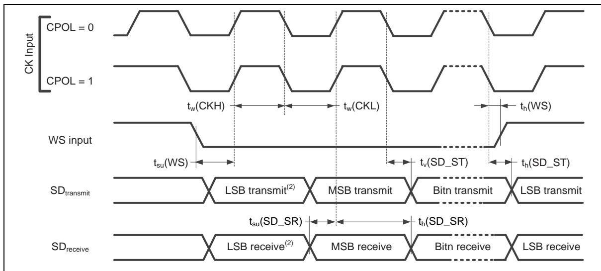
Figure 8.6-4 I<sup>2</sup>S Slave Mode Timing Diagram
