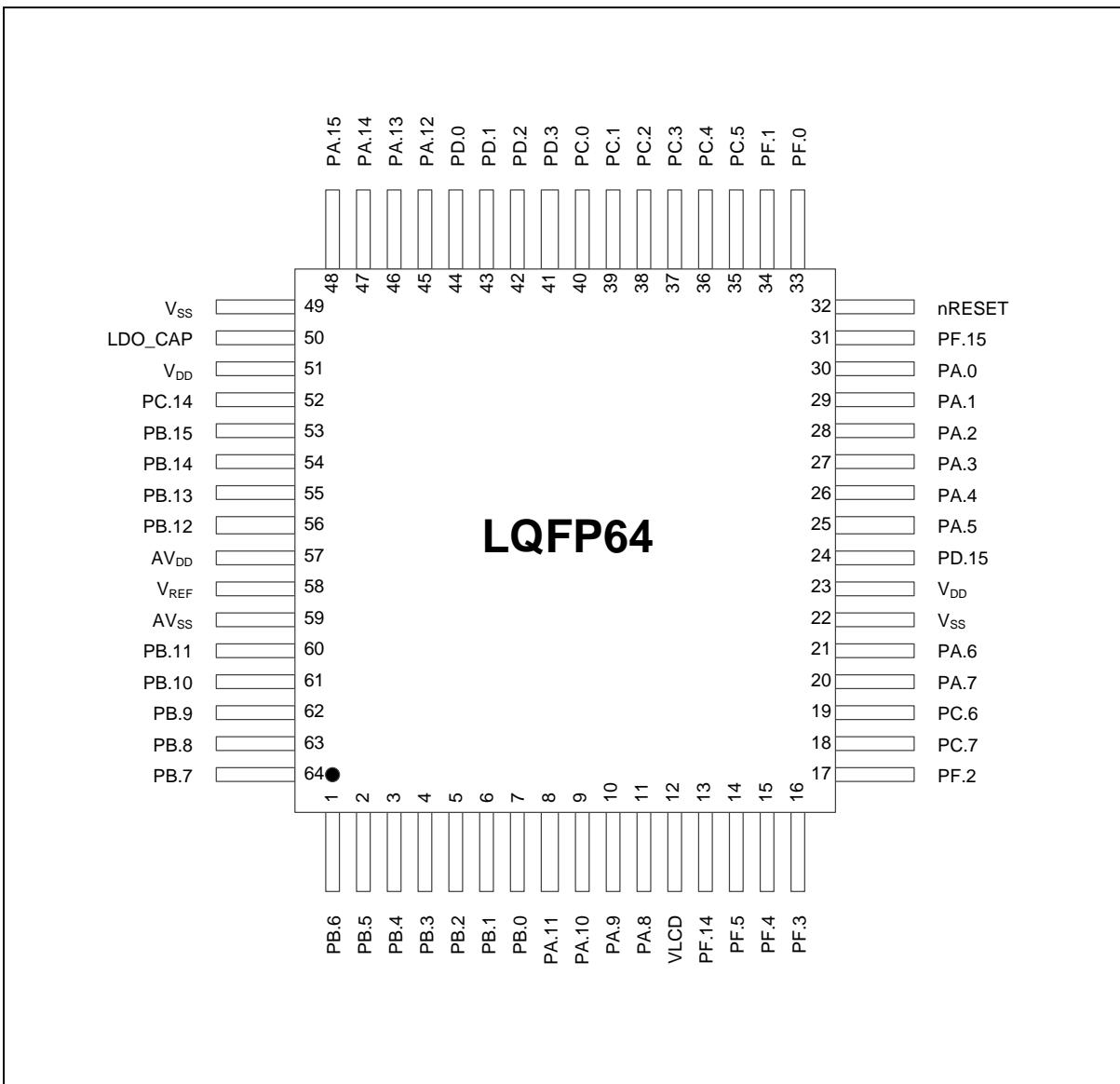
Figure 4.1-14 M256 Series LQFP 64-pin Diagram without V<sub>BAT</sub>
