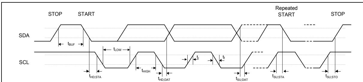
Figure 8.6-8 USCI-I<sup>2</sup>C Timing Diagram
